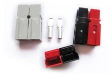
Anderson joint has no male and female shell design, it is fast and easy to install, has excellent electrical conductivity, and the shell can be inserted and removed up to 5000 times. All DC connections in the control box are connected using the Anderson connector.
