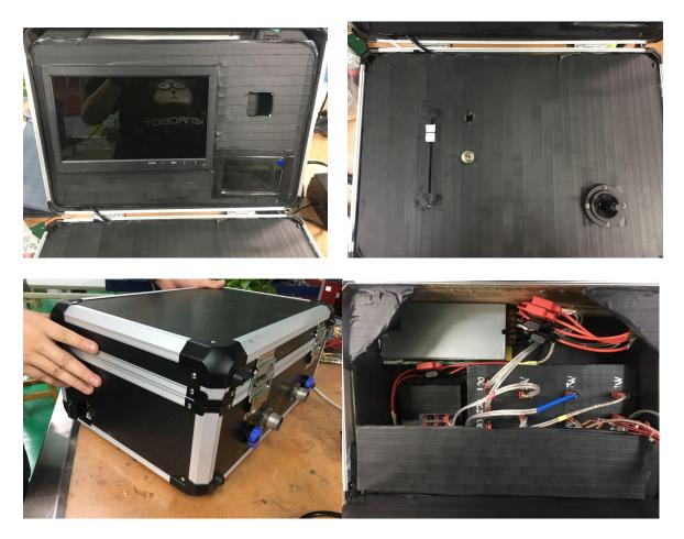
The control box consists of display panel, control panel and control circuit box. The display panel consists of two panels of 4.3-inch panel and 7-inch panel. The 7-inch panel displays the underwater panorama and 4.3-inch panel displays the arm Angle. Control panel is composed of rocker, slider, arm controller, rocker to control the robot around underwater, slider control robot floating sinking, arm controller to control arm.
