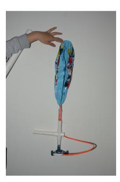
To retrieve the lost airplane's engine, we craft a device separate from our ROV and able to lift objects under the sea and bring them back to the ground. To achieve such task, we will use a manual air pump to inflate our lift bags through a pumping pipe. The heaviest object the ROV will lift during the competition weighs 45 N (which is approximately 4.59
