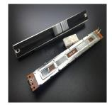
The motor is controlled by 10k direct - slip potentiometer. The motor speed is controlled by changing the resistance value. With 5k as the intermediate point, the resistance value slides from 5k to 0k, and the downward movement speed of the robot increases gradually. The resistance value is sliding from 5k to 10k, and the speed of upward movement of the robot increases gradually.
