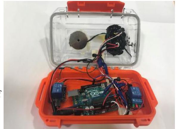
Figure 17: OBS Release Mechanism Internal Schematic
