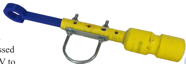
Figure 14: ADV Consist of Ballast, U Bolt, and Hook
