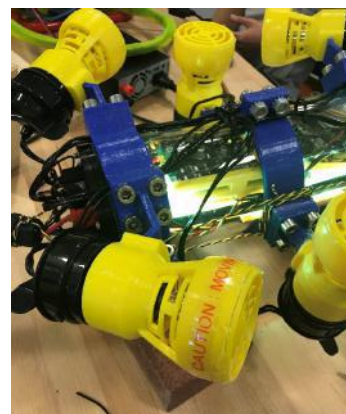
Figure 18: SPX 1250 GPH Bilge Pump with Safety Sticker
