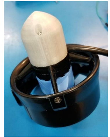
Figure 12 Final ESC housing installed
