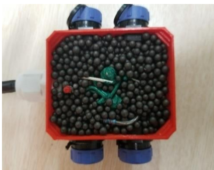
Figure 8 Universal Hub filled with foam balls before casting epoxy
