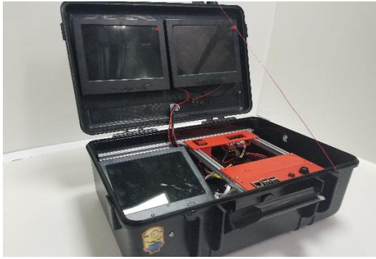
Figure 16 Control box with two monitors on top and one at the bottom. With the module racks on the right side,
