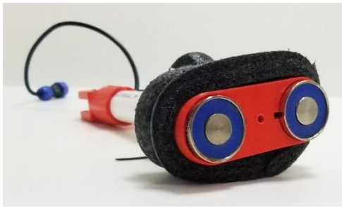
Figure 22 The Bi-electromagnet wrapped with foam
