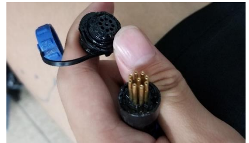
Figure 35 Broken socket due to the corrosion by petroleum jelly
