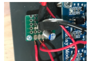
Figure 17 – 5V regulator for power
