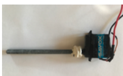
Figure 22 – Shaft that rotates the arm
