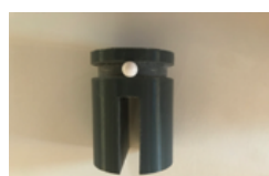
Figure 23 – Wheel piece with bearings
