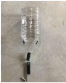
Figure 29 – Airbag to remove debris
