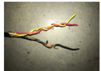
Figure 34 – Corroded wires due to rotating mechanism
