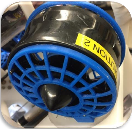
Figure 7: 1 of 6 BlueRobotics™ T100 Thrusters on ICE
