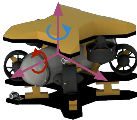
Figure 13: Thruster placement was carefully considered to afford the ROV five principal degrees of freedom: surge/sway/heave (violet), roll (red), and yaw (blue)
