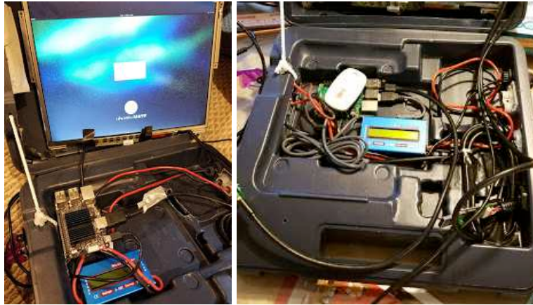
Figure 11: The Nemo topside control unit, including: (left) repurposed monitor and (right) electronics
