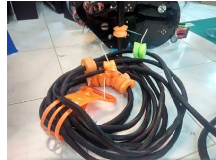
Figure 10: Tether management (Credit: Abyan)
