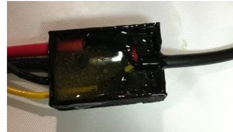
Sealing an epoxy box
