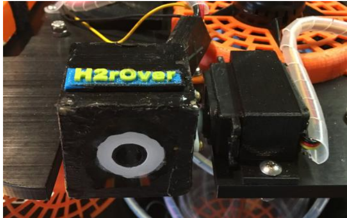
Primary front camera mounted to a servo
