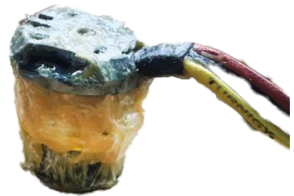
Brushless motor being waterproofed
