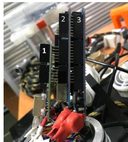
Figure 10. Boards: 1 – Ethernet Shield, 2 – Custom Shield, 3 – Arduino Mega
