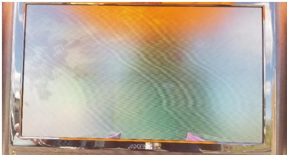
An example of camera interference that used to be a major issue in the Atlas. Having an onboard electronics housing prevents this.
