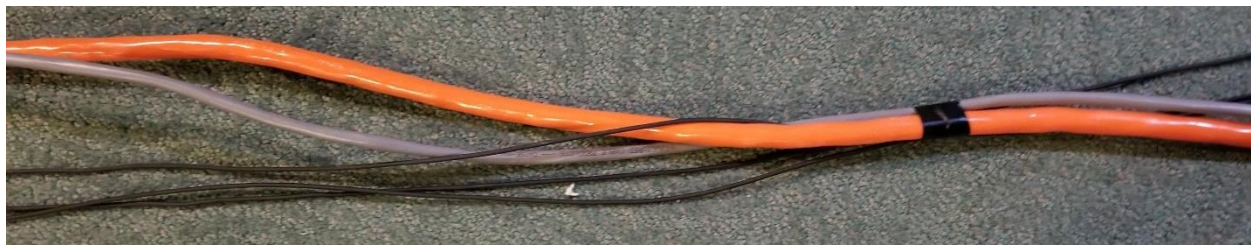
A section of tether. The orange cable is for power, the gray cable is for communications, and the black cables are for the cameras.
