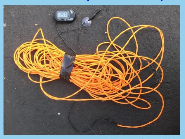
A temperature sensor with extended wire length that our ROV can take underwater.
