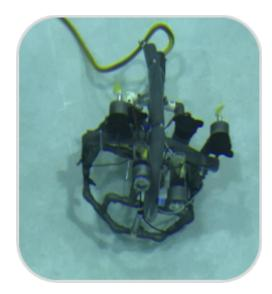
Our tether, included in the Barracuda ROV Kit, was also purchased from SeaMATE. It is 12.2 meters long, and includes a total of 13 wires. Eight of these are for our motors, two for each of the four. Three wires connect to our sensors, two inductive, and one temperature. The final two subjoin the cameras, one wire for each.
