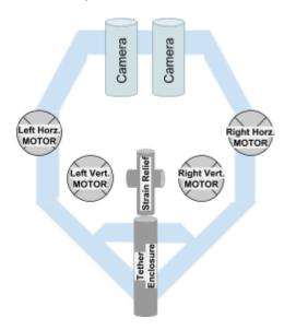
The final design of our ROV features four motors in mirroring positions on either side of the vehicle. Two of our motors face vertically, one up and one down, and the remaining two are placed horizontally, facing in the same direction. The reason for two of our motors facing the same way is because our ROV will mainly be driven forward, as opposed to side to side. Our unique motor placement easily serves the purpose of efficiency as well as maneuverability underwater.
