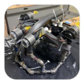
the monitor, the two cameras, as well as the inductive proximity sensor. The Arduino temperature reading circuit is powered by USB from a laptop. The thermistor runs through the Arduino.
