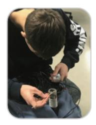
We have temperature and inductive sensors attached at the middle of our vehicle to allow us to gather ambient temperature data in the water and to detect metal objects for possible salvage inspection.
