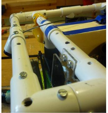
ROV in our chosen positon. The cylindrical shape of the pipes were desirable as it allowed us to attach 3D printed brackets to secure our pressurised tube and thrusters in position.
