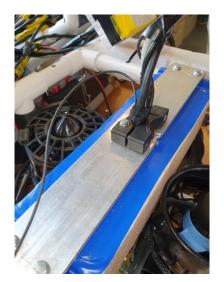
Mechanical clamp- To ensure the security of the tether we designed a clamp the keeps the tether up right and away from the thrusters, this also helps prevent the it from being tangled.
