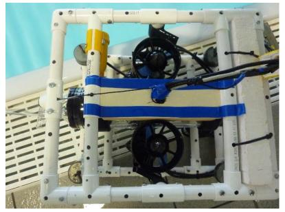
100g Weights – We used 100g weights because this allowed us to change our buoyancy in small increments. We installed metal poles and applied a screw thread on them to ensure that we could apply the weights and make sure they wouldn't fall off while
