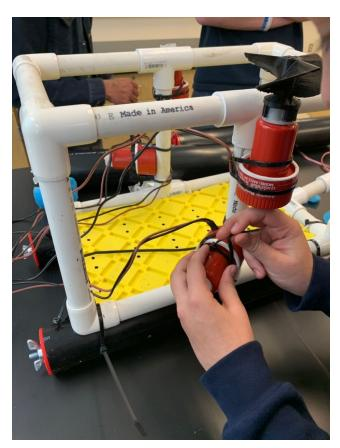
On the ROV, we have positioned 4 motors for optimal vehicle control. Positioned in the center, and one on each side, we have one set of motors pushing up and down to give us depth control. Next to the depth motors, we have forward and backward motors giving us the ability to move ahead or behind. Shrouded in a metal wire cage for safety, our motors are ready to move us to new places!
