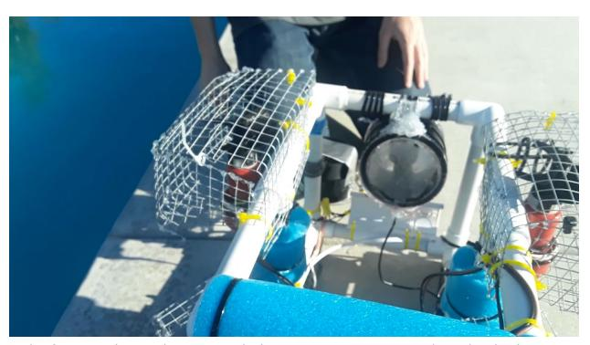
In the front, we have a larger, 8 inch diameter PVC pipe cut and sandwiched between clear plexiglass and sealed with waterproof silicone glue acting as our camera housing. This is attached to the top of the front of the ROV.
