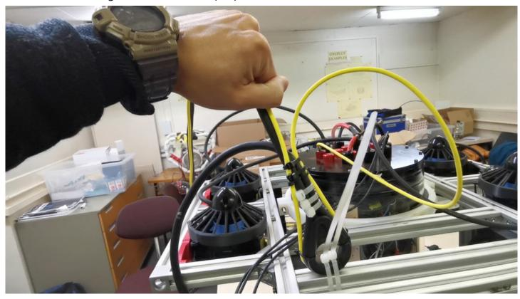
The tether leading to the ROV has proper strain relief.
