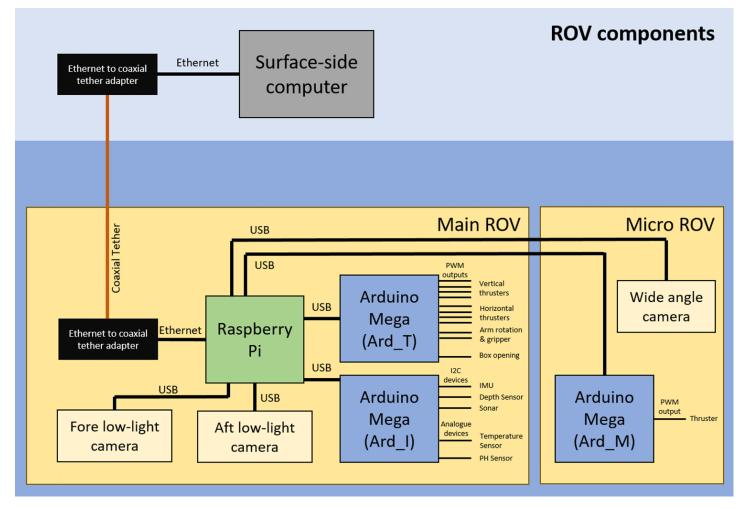
The middle-level layer, a Raspberry Pi, is the heart of the ROV. It runs on a modified Raspbian operating system and manages the data exchange between the surface and the lower-level electronics, as well as streams the videos from the cameras.
