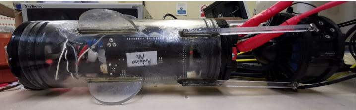
The mini-ROV comprises of an enclosure cylinder, fitted with a camera, lights, and a single T100 thruster. As the only objective required of the mini-ROV would be to explore
