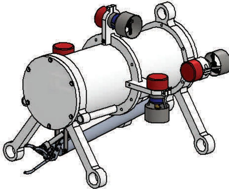
SolidWorks drawing of ROV Seadawg
