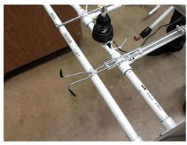
electrical tape for safety, which additionally also provided a better gripping surface due to a higher coefficient of friction. These hooks are intended to manipulate small objects, such as the CTA, the OBS pin, the OBS cable connector, bulkhead connector, as well as opening and closing the hatches of the BIA and the water column mooring platform.
