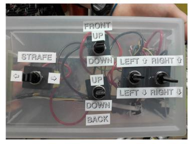
by spinning motors in opposite directions. The strafe motors, however, are each wired to one switch because there is no need for them to be independent of each other. Ultimately our ROV was designed to keep in mind safety, stability, and mission. Every component comes together to jointly address all the issues that compose this competition.
