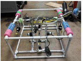
more reliable than trying to keep it airtight, where small leaks could cause it to gradually fill with water over time, altering our buoyancy. We attached pool noodles to the frame and tether to counter the weight of the motors, and attachments. Most of the flotation is attached to the top of the ROV, positioned far apart to the left and right, running lengthwise to limit the ROV's ability to inadvertently roll to the side, while preserving the ability to pitch forward or backward.
