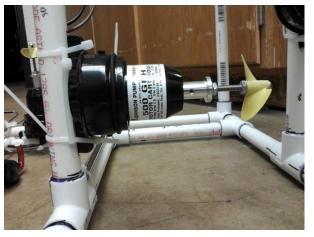
We learned from the 2012 MATE ROV competition that the ability to strafe would have been extremely beneficial for completing tasks. Having 2 motors dedicated to strafing allows the ROV to maneuver around objects without having to turn. This process allows us to always have the objects in our frame of view. The strafing motors are each mounted to vertical pillars on the centerline of the ROV, with each motor facing outward while still wholly contained within the frame. The low placement
