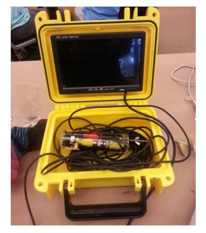
Dry boxes make wonderful holders for the camera system if you do not have a convenient place to mount the monitor. The cable and camera will also fit nicely into the box.
