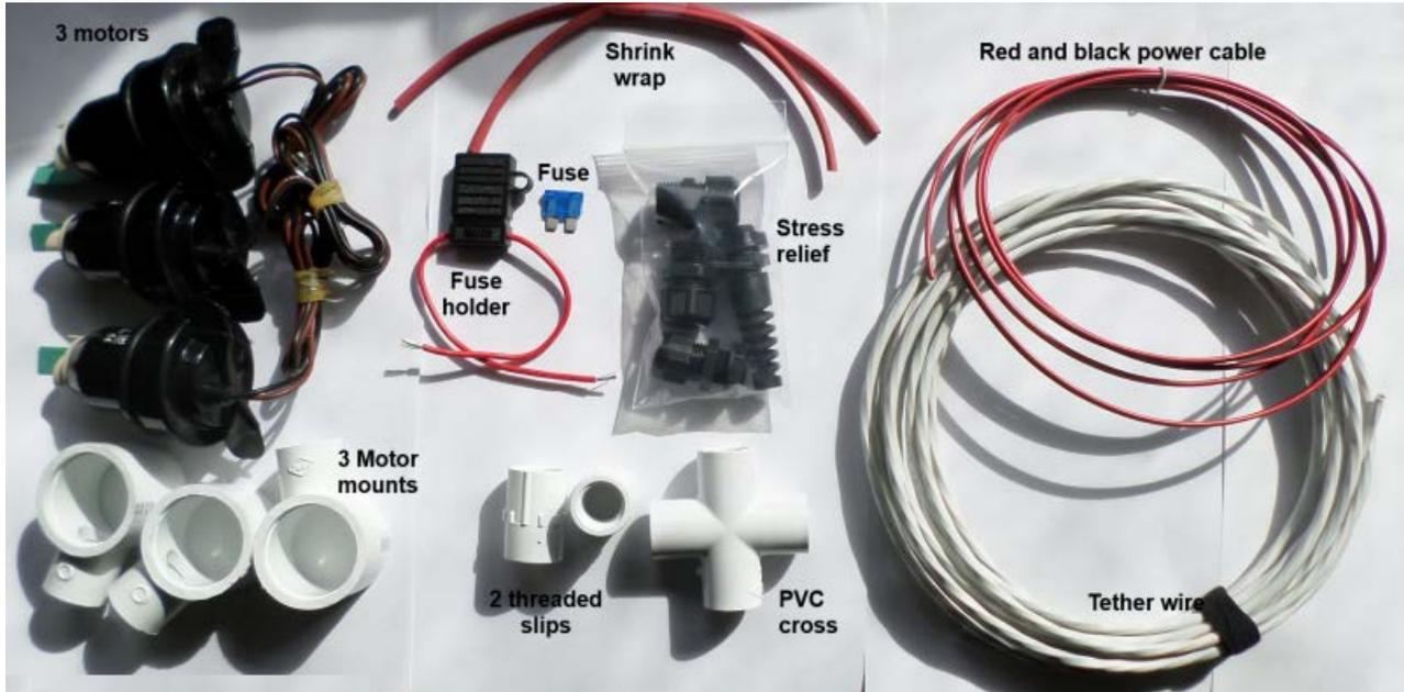
**Photo above:** Three bilge pump motors, three PVC motor mounts, two lengths of shrink wrap, one fuse holder with fuse, stress relief bag with 3/8-inch dome long, 3/8-inch dome short, and two 1/2-inch dome short stress reliefs, two threaded PVC slips, one PVC cross, 8 feet of red and black power cable, 25 feet of 18 gauge, six strand tether wire.
