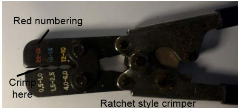
Give the wire/crimp connection a tug when the crimping is complete to ensure a secure connection. If the wire comes out when you tug on it, the connection was not good. Use a new red ring terminal (throw out the old one) and try again. A few extra terminals are included in AngelFish kit, as is some extra 18-gauge wire, to use when crimping problems occur.
