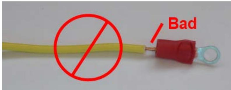
***Very bad connection. The exposed wire outside the plastic covering can cause a short circuit.***
