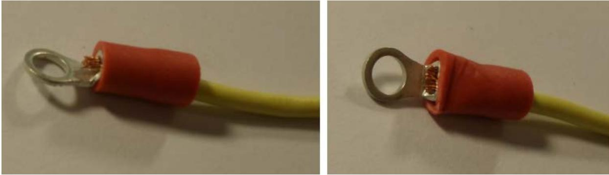
**Copper wire emerging 2 mm beyond the metal ring. Metal ring securely crimped over copper wire.**
