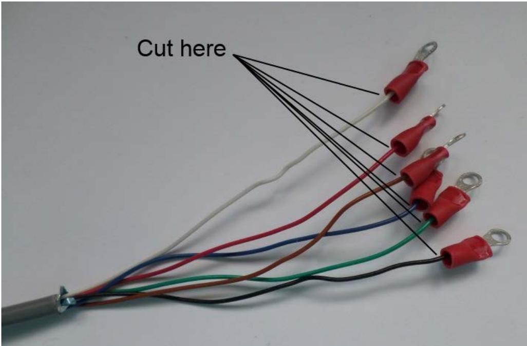
4. Cut the two terminal ring connectors from the end of the power wires. Again, cut as closely to the terminal ring connector as possible to minimize loss of wire.
