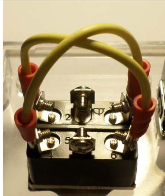
*Wires connecting post #1 to #6, post #3 to #4.*
