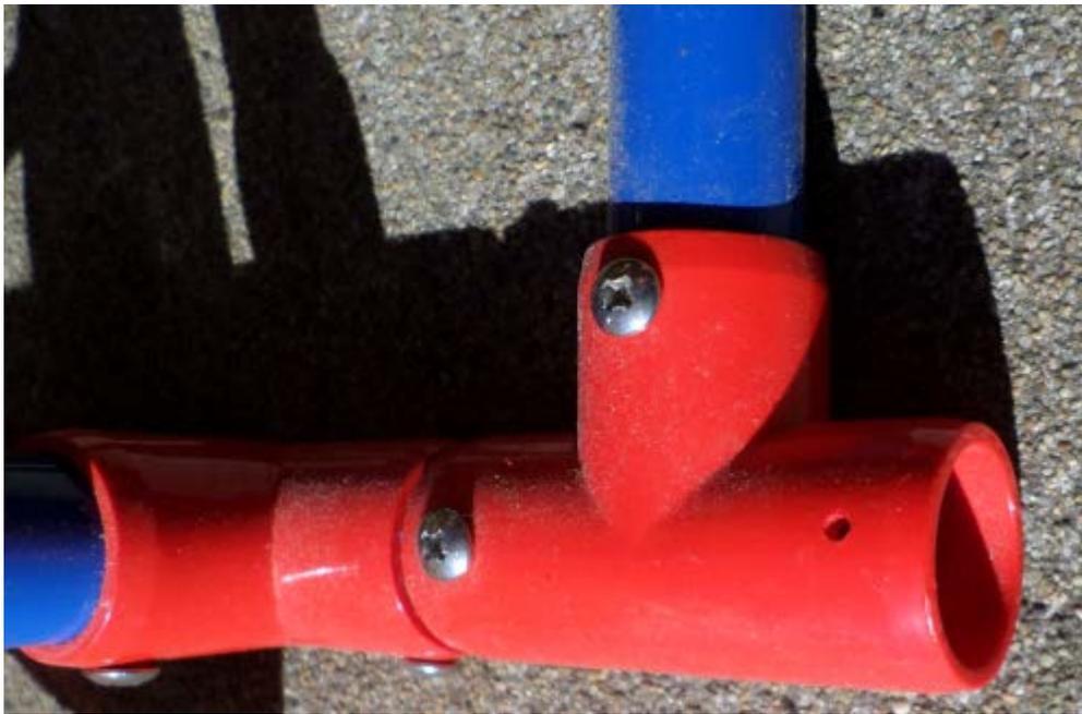
*Colored PVC frame screwed together. Also note the PVC tee used to allow water to flow in and out the frame of the vehicle.*
