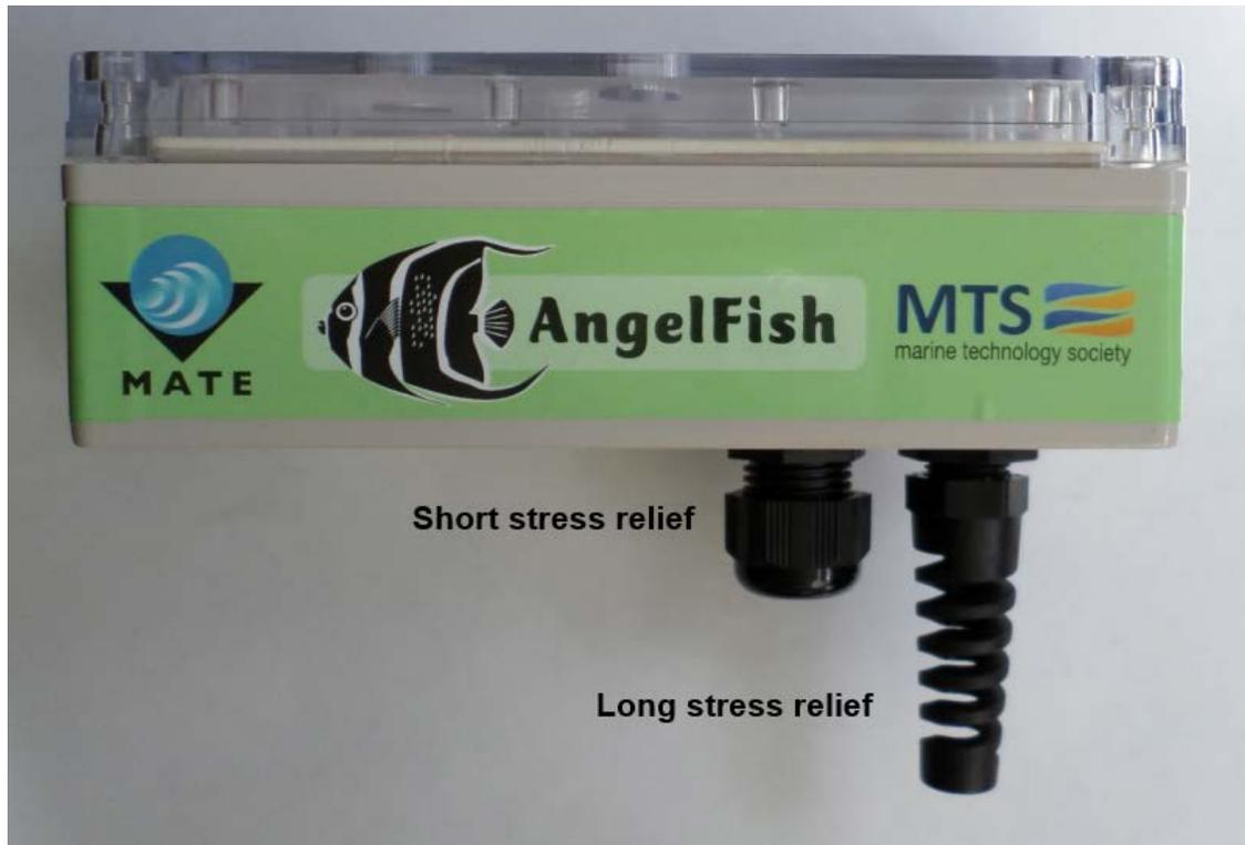
*Side view of control box with both stress reliefs installed.*
