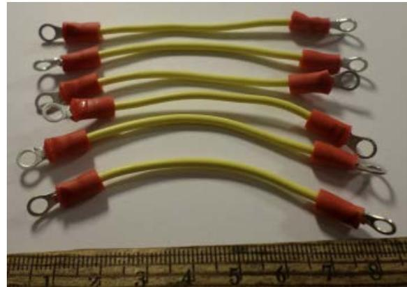
When crimping the ring terminals onto the end of the wire, it is important to get a secure, metal to metal connection. If the ring terminal is not secured properly to the bare metal wire, electricity may not flow through the connection and your controller will not work. To make a secure crimp connection:
