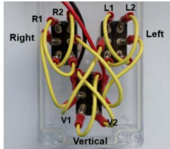
5. Carefully unscrew R1 on the right switch (Note that this may NOT be post #1). This post should have part of the "X" on it. The right switch is black and white tether wires, unless a different color configuration is used. Attach the black tether wire and the removed "X" wire to this post. Tighten the screw to secure both ring terminals to the post.
