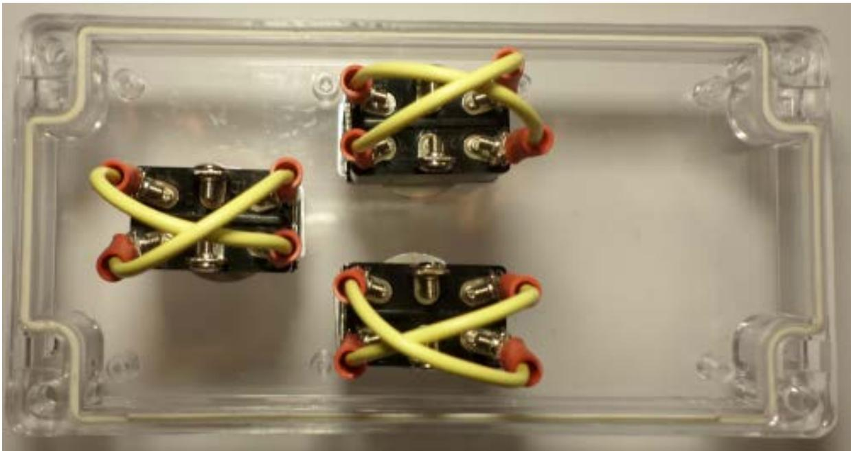
*The three switches with "X" wires on the back of each.*
