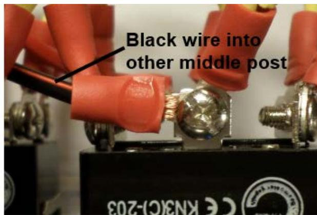
Once both the red and black wire are secured to a switch, pull the any excess power wire back out through the small stress relief. Tighten the small stress relief nut over the threads to secure the power wire in place.
