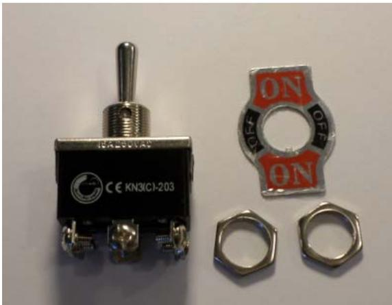
*Disassembled components on the switch*
