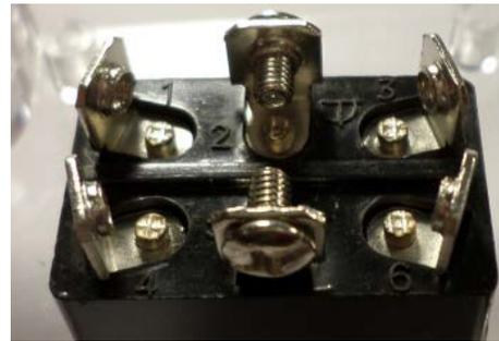
***Screws on post 1, 3, 4 and 6 removed.***
