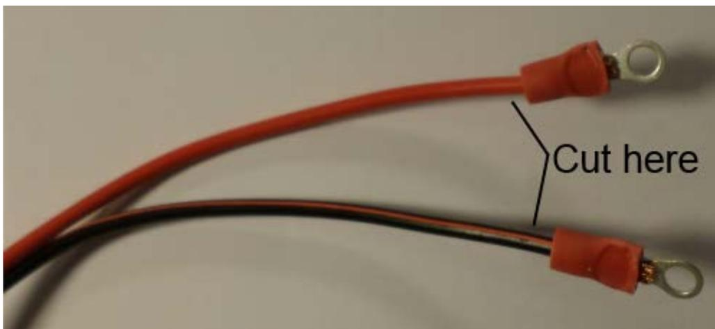
The AngelFish control box replacement kit includes new 18-gauge wire to construct the X's power jumpers on the back of each switch, and new terminal ring connectors to crimp on the end of the wires.
