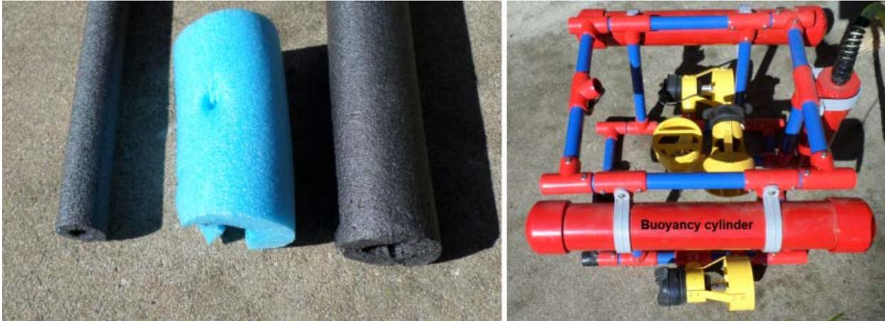
*Photo above (left): Soft foam flotation in various sizes, all will compress under pressure. The ROV on the right uses hard buoyancy cylinders made out of 2-inch PVC pipe with end caps.*
